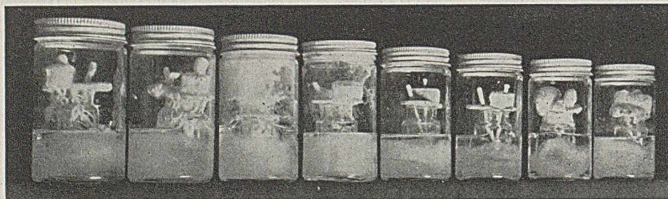
FIGURE 6. ASSAY OF WORTHLESS PRESERVATIVE AT MAXIMUM CONCENTRATION Fungi in duplicate, left to right, Lenzites trabea , U-10, Fomes roseus , and Lentinus lepideus
