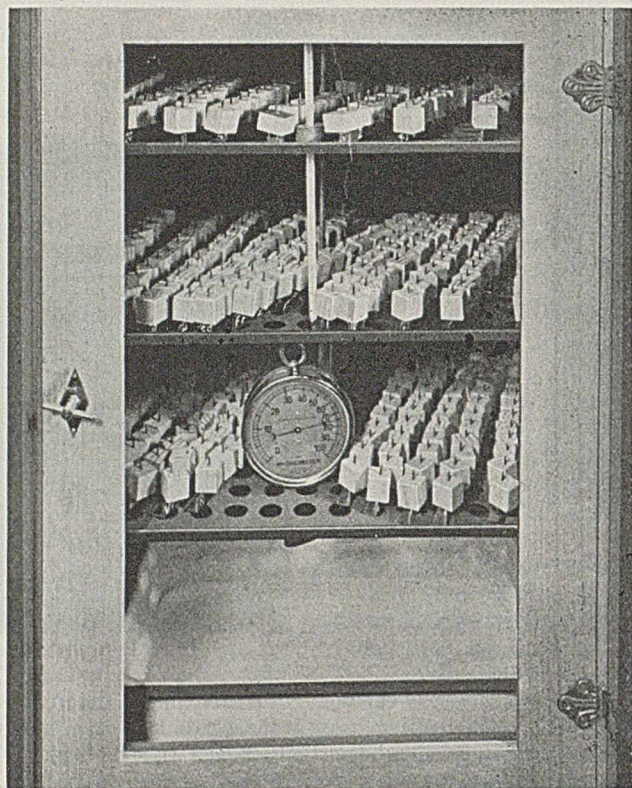
FIGURE 4. CONSTANT-HUMIDITY CHAMBER FILLED WITH TEST BLOCKS
