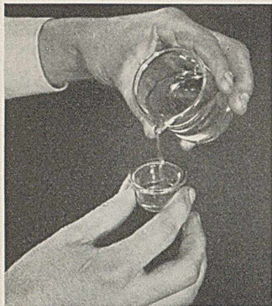
Sample cup is quickly filled. Only a 5 ml sample of solution is necessary for accurate determinations.
