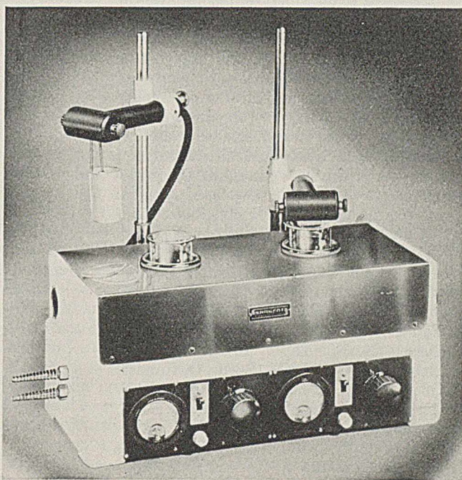
FIGURE 2. INSTRUMENTAL SIMPLIFICATION RESULTING FROM SOLENOID STIRRING
