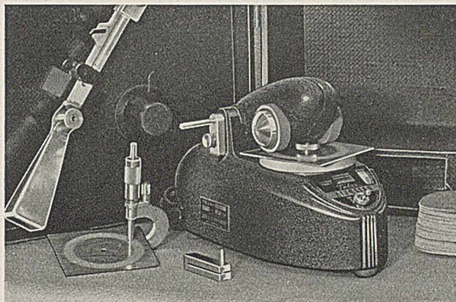
Taber Type J Abraser Testing a 4" sq. Specimen
