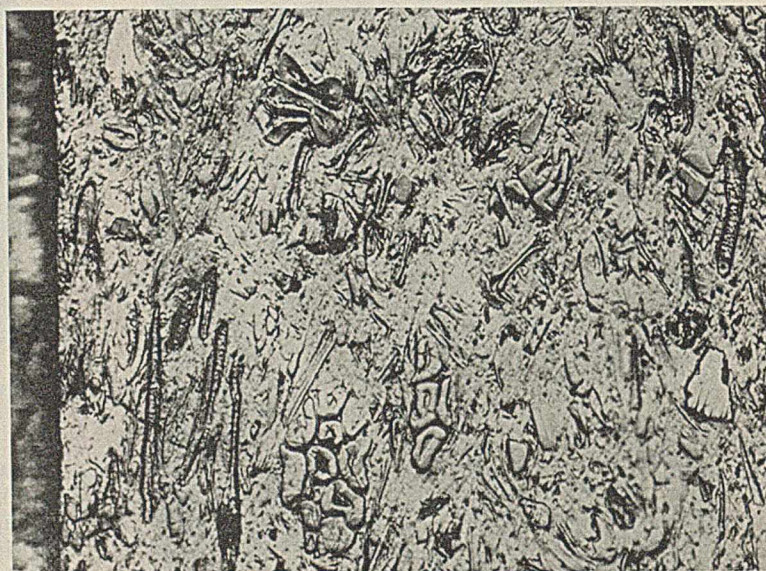
FIGURE 14. PHENOLIC RESIN WITH GROUND WOOD AND MINERAL FILLERS POLISHED CROSS SECTION ( \times 250 )
