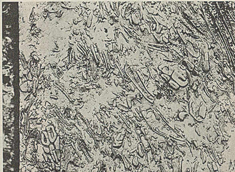
FIGURE 13. PHENOLIC RESIN WITH WOOD FLOUR AS FILLER, POLISHED CROSS SECTION ( \times 250 )
