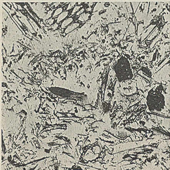
FIGURE 15. HEMP HURDS IN MOLDED PHENOLIC RESIN, POLISHED CROSS SECTION ( \times 250 )
