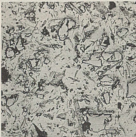
FIGURE 20. TALC IN MOLDED PHENOLIC RESIN, POLISHED CROSS SECTION ( \times 250 )
