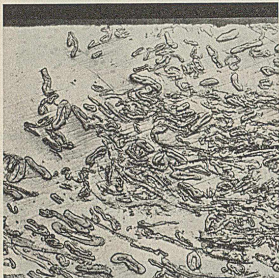
FIGURE 11. PHENOLIC RESIN WITH PAPER PULP FILLER ( \times 250 )
