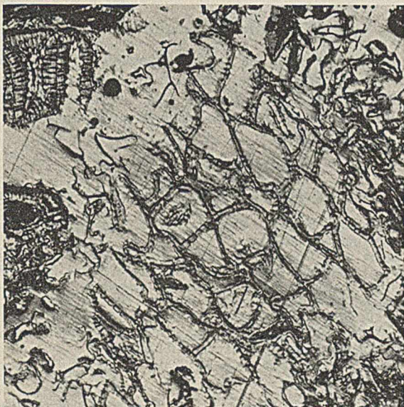
FIGURE 16. CORK IN MOLDED PHENOLIC RESIN, POLISHED CROSS SECTION ( \times 250 )
