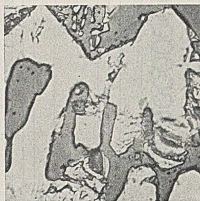
FIGURE 5. SLAG ( \times 1000 ) Polished section, showing magnetite crystals in a matrix of ferrous akermanite
