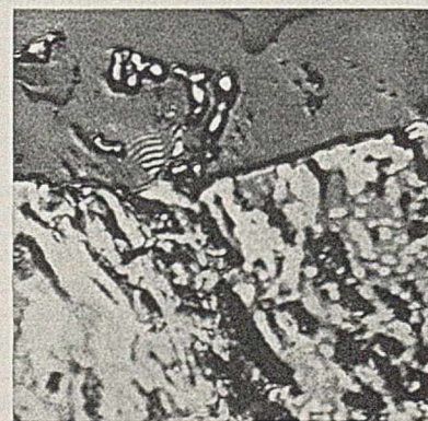
FIGURE 7. CRUCIBLE WALL-SLAG INTERFACE ( \times 1000 ) Polished section. Dark area is slag.
