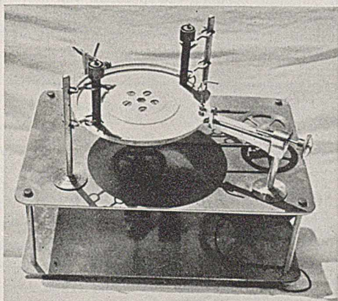
ABRASION MACHINE ONLY, SEEN FROM ABOVE Clear view of specimen holders and removable wax plate
