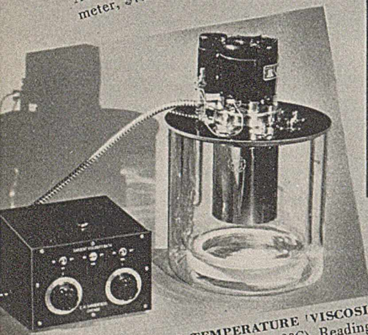
SARGENT HIGH SPEED HEAVY DUTY ELECTROLYTIC ANALYZER —Operating with current densities as high as 10 amperes, it reduces time formerly required for deposition by as much as 60%. Electrolyte agitated electromagnetically—mechanical, stirring mechanisms eliminated.
