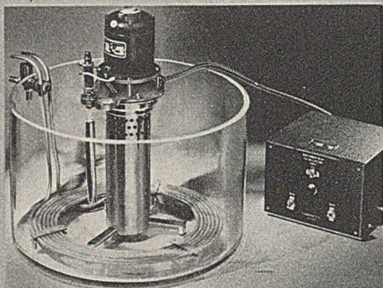
SARGENT CONSTANT TEMPERATURE WATER BATH —Guaranteed accuracy of regulation and uniformity, 0.01°C. Range, up to 60°C. Immersed objects fully visible through walls of container.
