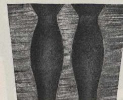
Vertical cross-section of HR-108 two-hole stopper, showing Hough fusiform openings.
