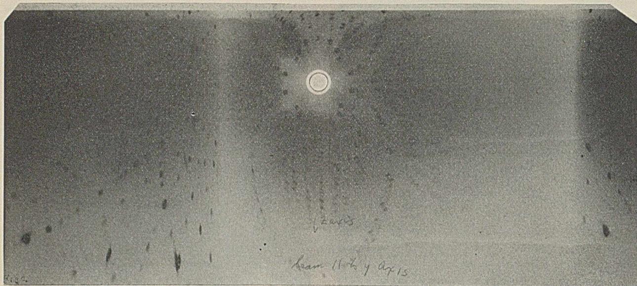
FIGURE 91. PATTERN OBTAINED IN CYLINDRICAL CASSETTE MOUNTED ON UNIVERSAL SPECIMEN MOUNT
