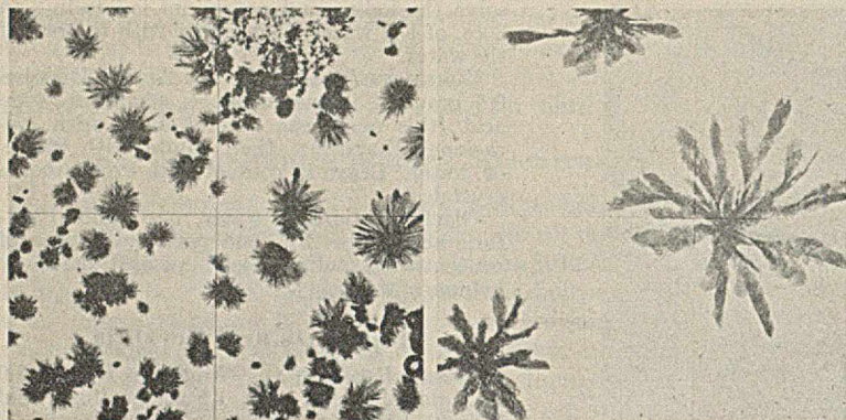
FIGURE 4. CINCHONIDINE PLATE CRYSTALS, WITH ORDINARY LIGHT, REAGENT C-2 (left); CINCHONINE-CINCHONIDINE MIXED CRYSTALS, REAGENT C-1 (right)
