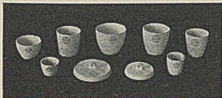
If the crucible is placed in a bath of concentrated hydrochloric acid for several hours, thoroughly rinsed, and then dried, filtration is improved very much. Possibly minerals from the materials ashed in the crucible, such as animal feeds, have filled the pores of the crucible and hence cut down the rate of filtration. The acid treatment thus dissolves the mineral matter and opens the pores of the crucible again.
