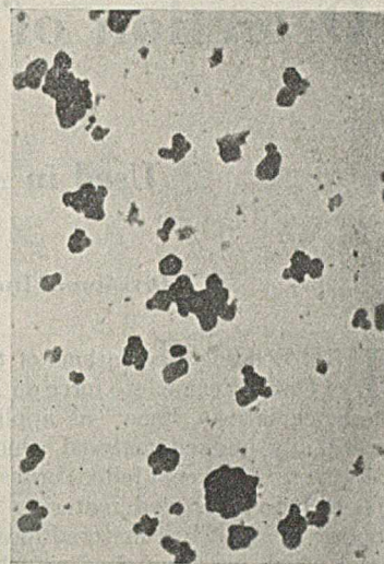
FIGURE 8. ELECTRON MICROSCOPE PHOTOGRAPH OF \text{TiO}_2\text{-II} ( \times 14,600 )
