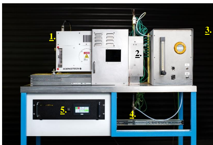
Fig. 3.7. Research stand for a study on the solar pyrolysis of waste biomass (1- xenon arc lamp, 2- insulated copper reactor, 3- data acquisition system container, 4- reactor outlet, liquid fraction condenser, 5- arc lamp power supply).
