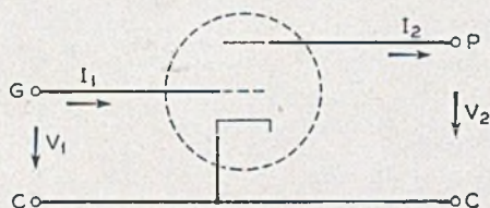
Fig. 16—Current-voltage relations for the grounded cathode triode.
