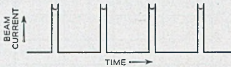
Fig. 12.2—If the electron beam were bunched into pulses short compared with a cycle, the peak value of the component of fundamental frequency would be twice the d-c current I_0 .
