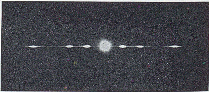
Fig. 5.—Spectrum formed by the grid of the 1553 microwave triode.
