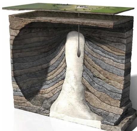
Fig. 2.4 Salt domes are considered a proper environment for final storage in Germany [13]
