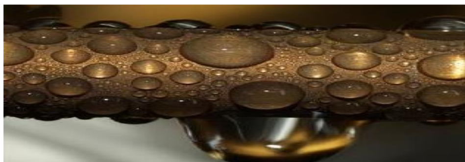
Fig. 4.6 Drop-wise condensation on Nano structured Plain Tube
