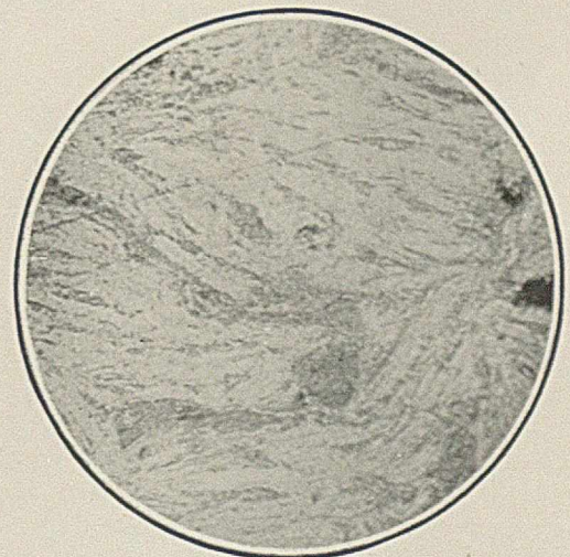
Fig. 31. \times 65 . Carbon from coarse natural graphite. Relief polish.
