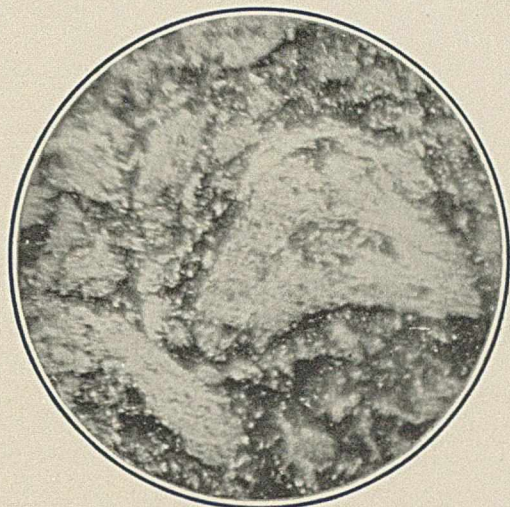
Fig. 3. \times 200 . Carbon sample showing structure and individual grains. Heat-etched.
