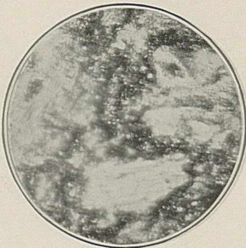
Fig. 24. \times 200 . Sample containing petroleum coke and artificial graphite. Heat-etched.
