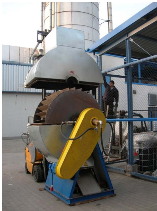
Fig. 4.2 Gasification/pyrolysis reactor under construction
