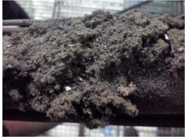
Fig.3.4. Ash deposit collected during DS0 900°C tests - close-up image, visible sintered ashes and agglomerates .
