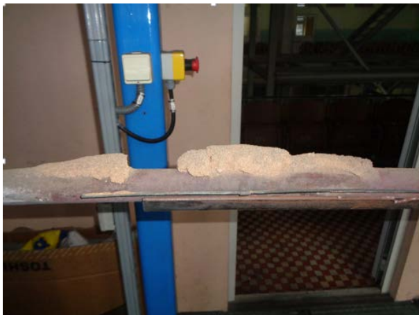
Fig.3.1. Ash deposit collected during DS4 900^{\circ}\text{C} tests. Part of the deposit has automatically dropped out.
