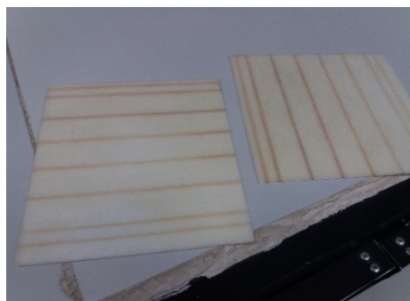
Fig.1 (a) Sulfonic group Cationic resin (b) Ammonium group anionic resin (b) resin coating on membrane (d) set of prepared dried membranes
