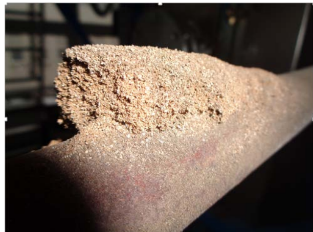
Fig.3.2. Ash deposit collected during DS4 900^{\circ}\text{C} tests - close-up image, powdery deposit.
