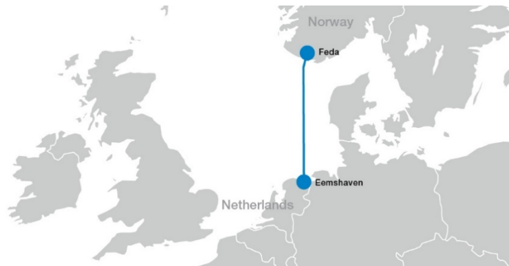
Fig. 3.2. NorNed HVDC submarine cable line [16]
