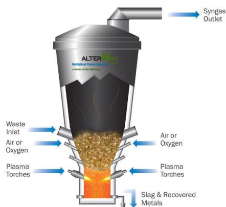
Rys. 4.2. Schemat reaktora Alter NRG Westinghouse Plasma Corporation [20]
