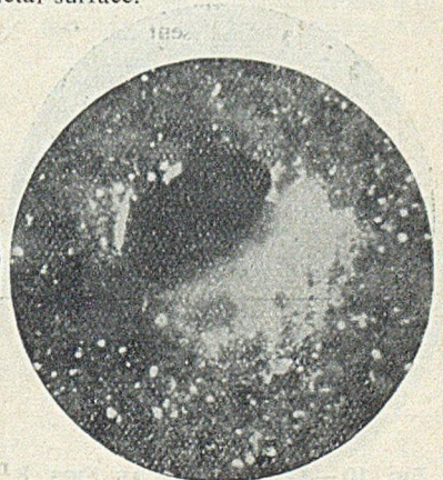
FIG. 6.—SAMPLE AFTER 2 MIN. IN THE FURNACE. SINTERING IS IN PROGRESS.
