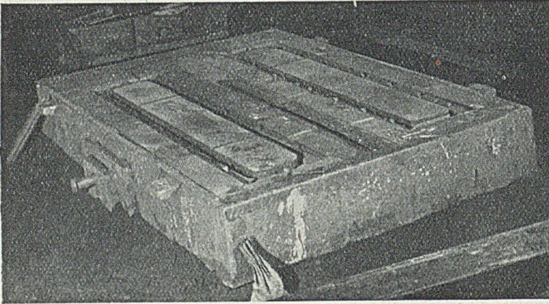
FIG. 21. — MOUTHPIECE HALF-MOULD MADE ON A MACHINE.
