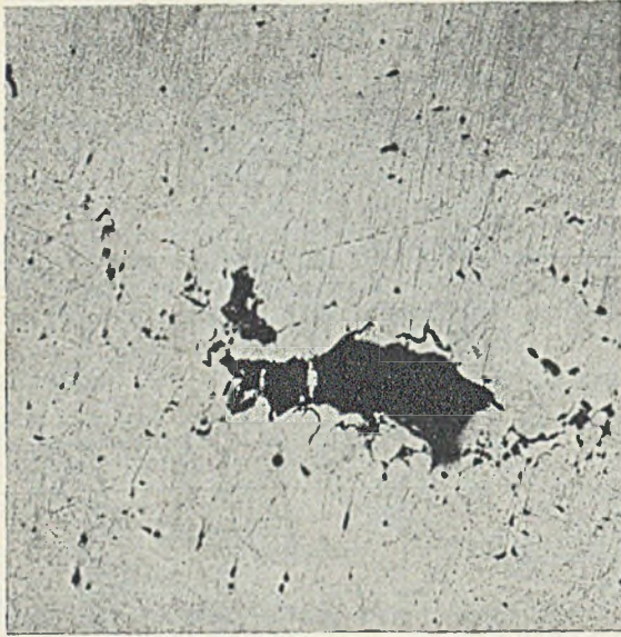
FIG. 19.—GAS HOLE IN ALUMINIUM ALLOY SURROUNDED BY MICROPOROSITY.
