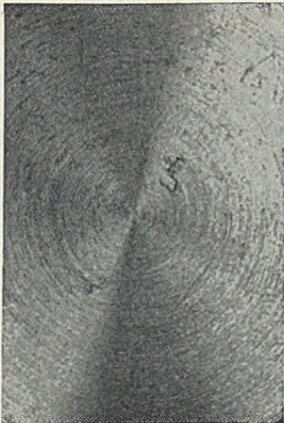
FIG. 15.—ABSENCE OF PINHOLE FORMATION AT 760 DEG. C. IN 40E ALUMINIUM ALLOY. ( \times 1.12 )
