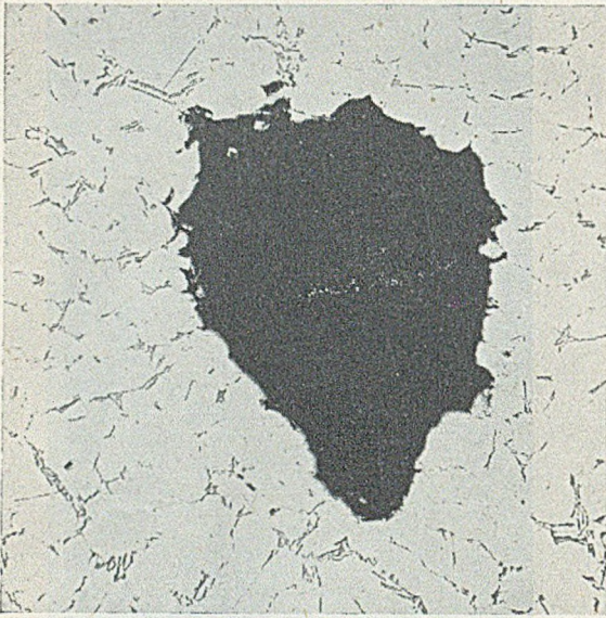
FIG. 17.—SINGLE PINHOLE WHICH IS TYPICAL OF THIS DEFECT IN ALUMINIUM ALLOYS.
