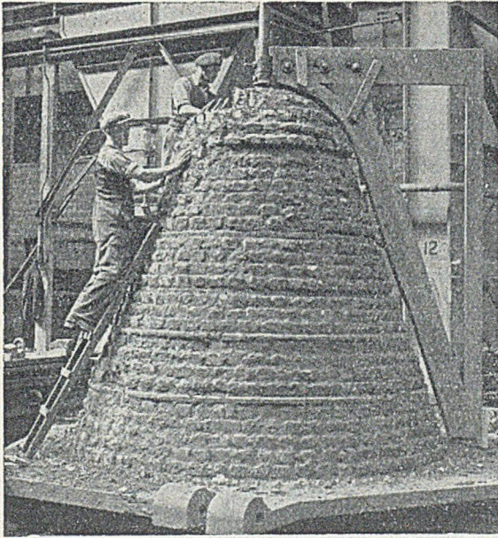
FIG. 2.—First Stage of the Pin and Strickle Board Technique of preparing a Core for a Pollock-type Slag Ladle.
