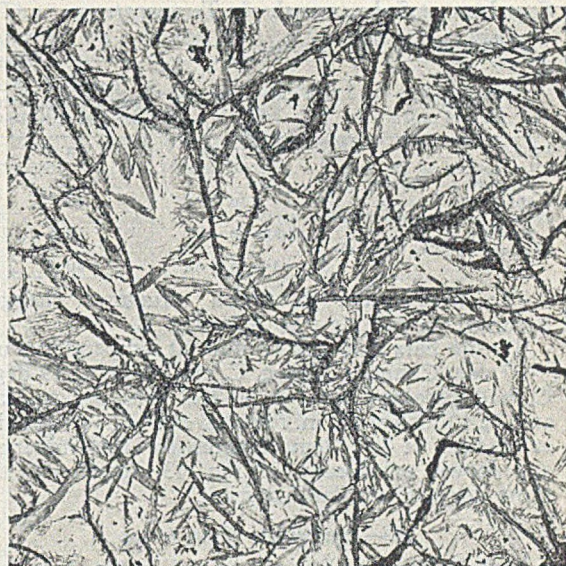
FIG. 16.—Same Material after Treatment at -55 deg. C. Etched \times 100 .
