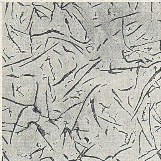
FIG. 14.—Structure of Nickel-Copper-Chromium Austenitic Iron W335 in the As-cast state. Graphite Flakes in a Matrix of Austenite with a little Carbide. Etched in 4 per cent. Picral \times 100 .
