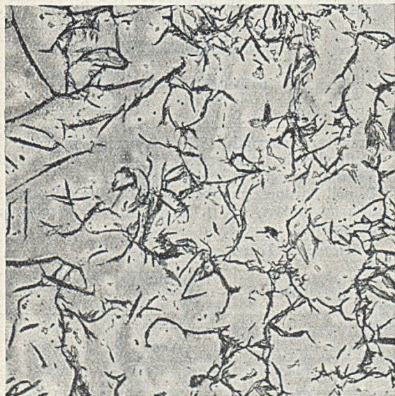
FIG. 15.—Same Material as shown in Fig. 14, after Treatment at -20 deg. C. Etched in 4 per cent. Picral \times 100 .
