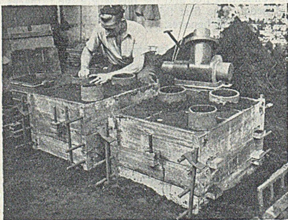
FIG. 3.—Cast-aluminium Moulding Boxes made on the Premises. The Moulds are for Tee Castings for Hydrovac Equipment, Pattern shown in the Background. Note the Adjustable Box Clamps.
