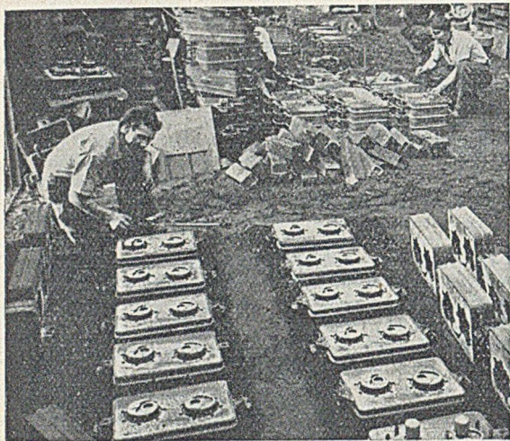
FIG. 1.—Section of the Iron Foundry. In the Fore-ground are Moulds for Steam Valve Covers.
