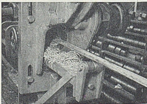
FIG. 5.—Drawing the Straightened Bar through a Sharp-edged "Scalping" Die.
