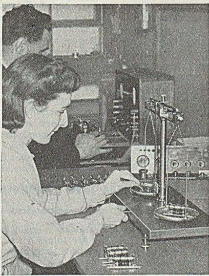
Weighing and level calculation for special level switches
