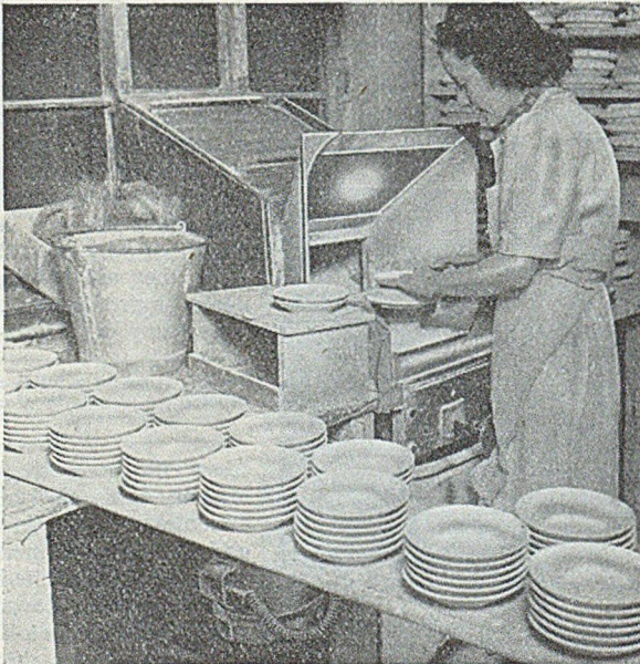
After drying, certain articles go to trowing machines where the rough edges are removed
