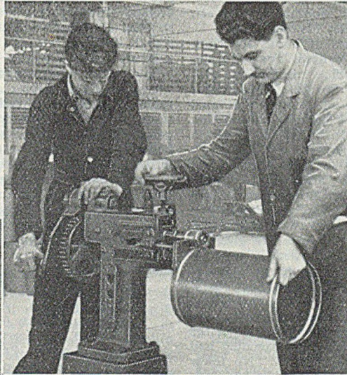
Swaging a case for a 1½-gal. storage heater
