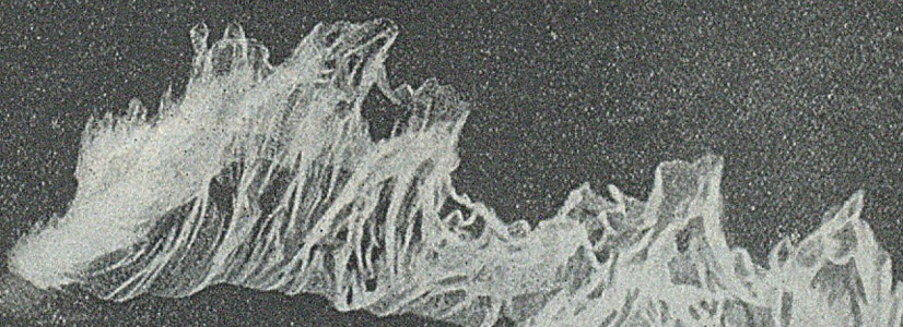
The first 1,000,000 Volts Power Frequency Arc in Britain produced in the Ferranti Laboratories in 1925.
