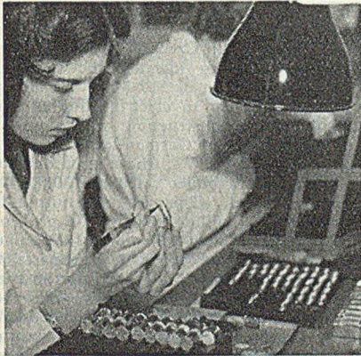
Above: Assembling the cage of a five-grid type battery valve. Right: Welding the completed cage of a mains valve to its base
