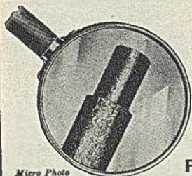
Micro Photo of hair actually turned on a Pultra Lathe.
