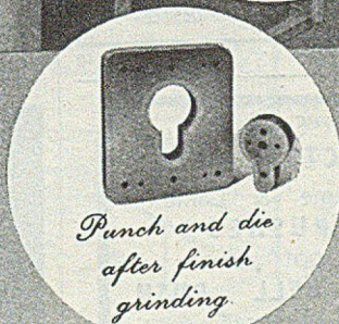
Punch and die with weld deposit of tool steel
