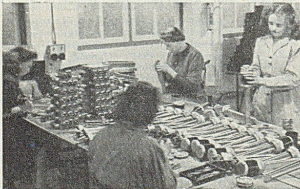
Assembling immersion heaters at C. H. Blackburn & Co.'s Stellex Works, Calne
