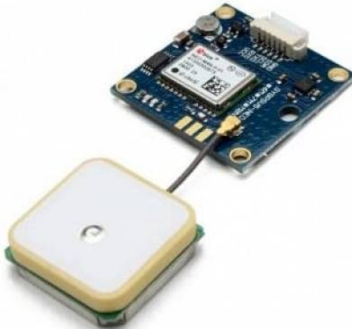
Figure 96. A GPS receiver module with ceramic antenna
