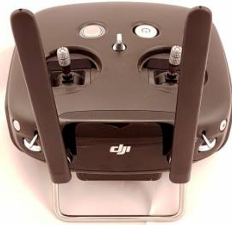
Figure 120. Additional switches (located on the figure close to the antennas) that control AUX channels 5+
