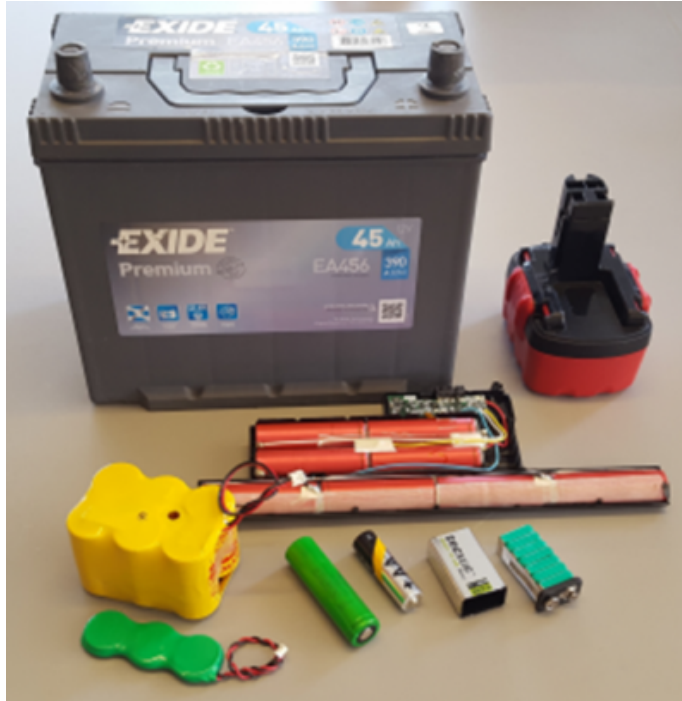
Figure 22. From top left: car 12 V lead-acid battery (6 cells), cordless drill 14.4 V NiCd battery (12 cells), laptop 14.4 V Li-ion battery (8 cells), special-purpose medical equipment 7.2 V NiCd battery (6 cells), memory back-up 3.6 V NiMH battery (3 cells), 18650-size Li-ion 3.6 V battery (single cell), generic AA size 1.5 V primary battery (single cell), disassembled 9 V NiMH battery (7 cells).
