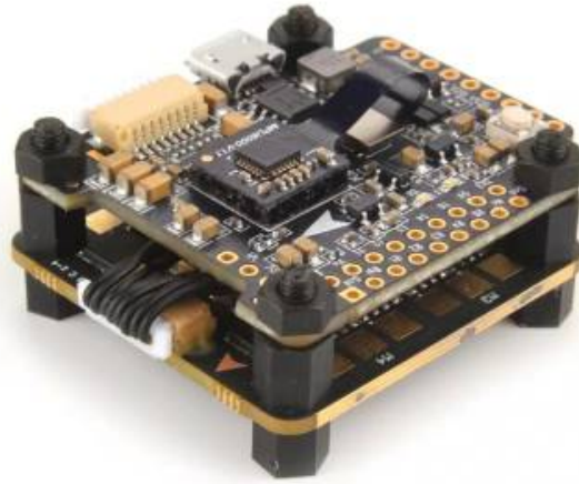
Figure 111. Stacked FC, here Kakute Holybro with brushless ESC for quadcopter
