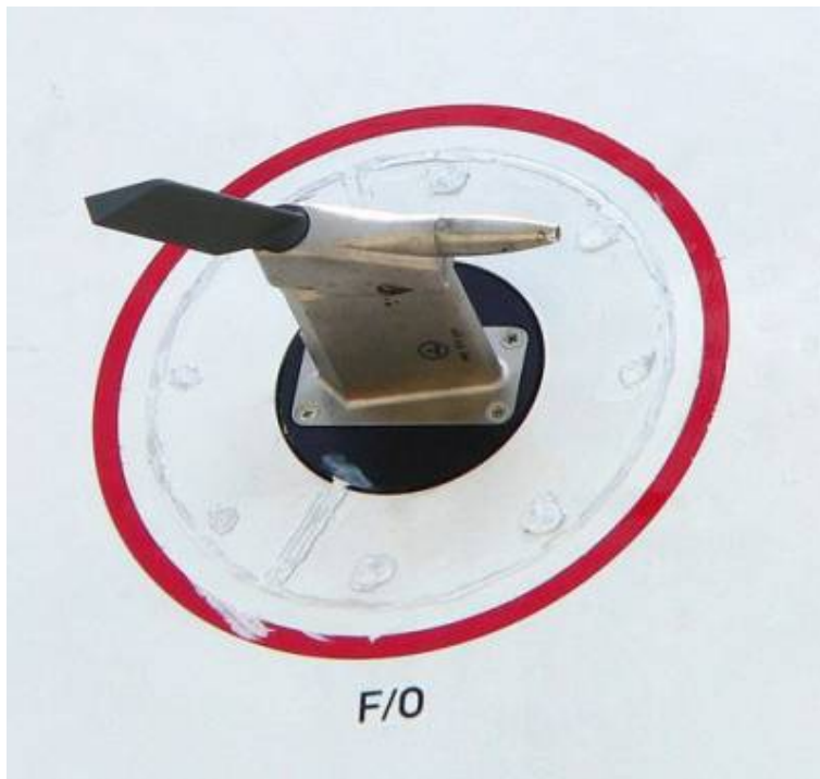
Figure 93. Full scale pitot tube with heating system to prevent ice clogs
