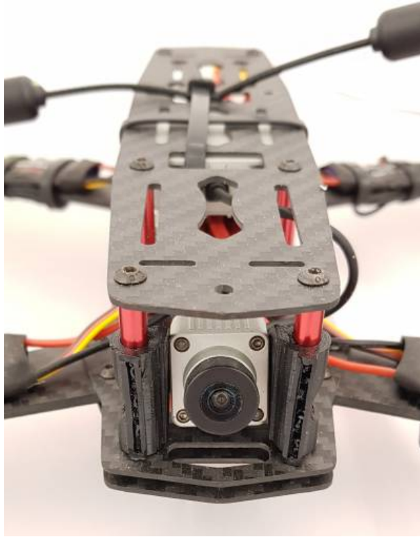
Figure 130. FPV racing drone camera, no stabilisation
