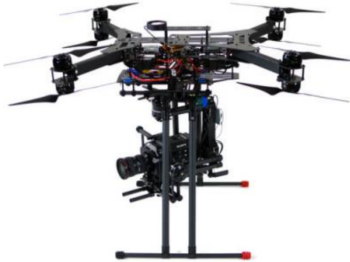
Figure 124. Heavy lifting cinematic drone with professional movie camera onboard (photo courtesy BPhotoVideo.com)
