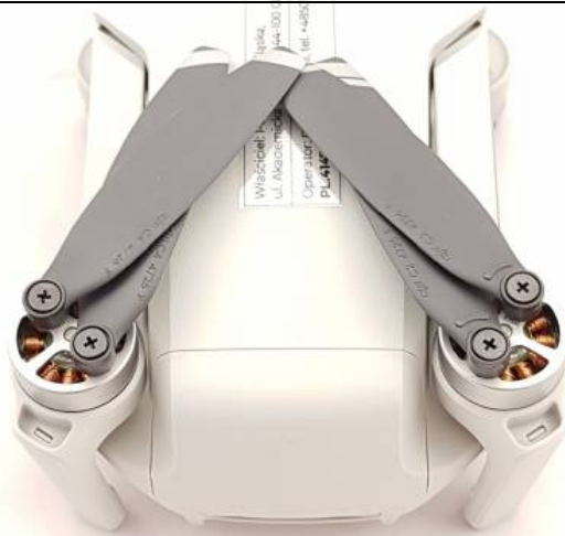
Figure 107. Planar foldable propellers, for transportation, DJI Mavic Mini
