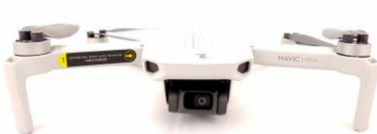
Figure 129. Front-mounted camera with stabiliser and possibility to tilt it
