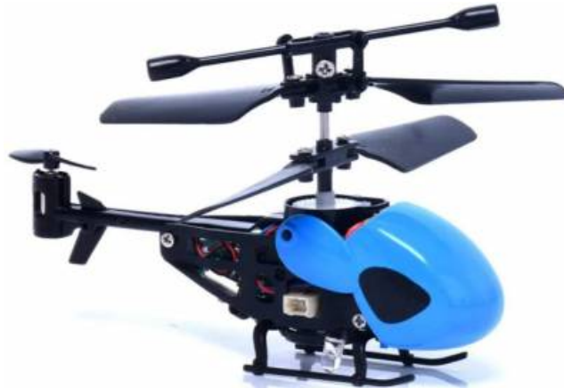
Figure 44. Miniature RC helicopter with coaxial, counterrotating two main rotors
