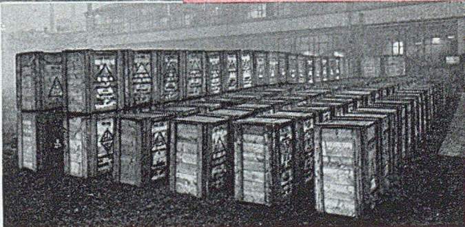
Batch of 120 hermetically sealed stoneware container transformers ready for despatch
