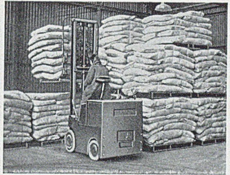
Above : This exceptionally large battery truck has four speeds ; Lansing Bagnall. Right : Palletization and the fork truck are parallel developments ; Ransomes, Sims & Jefferies (photo courtesy W. T. Glover & Co.)
