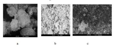
Fig. 1. SEM – images of plate-like sorbent surfaces, obtained from calcium silicate powders by standard synthesis (a), with PVA addition (b), by microemulsion method with quaternary ammonium base (c)
