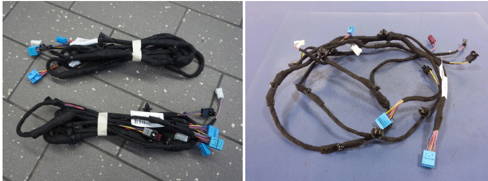
Fig. 3.1. Mercedes S-class W222 Door Harness
