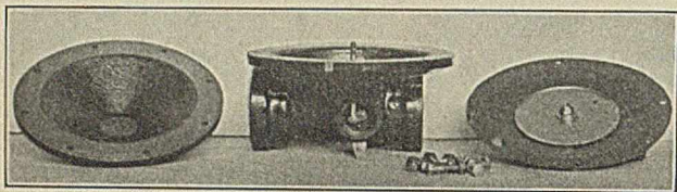
FIG. 46—AIR PRESSURE REGULATOR PARTLY ASSEMBLED, SHOWING AT THE CENTER CONNECTING ROD AND CRANK FOR ACTUATING THE DAMPER BY THE DIAPHRAGM MOVEMENT
