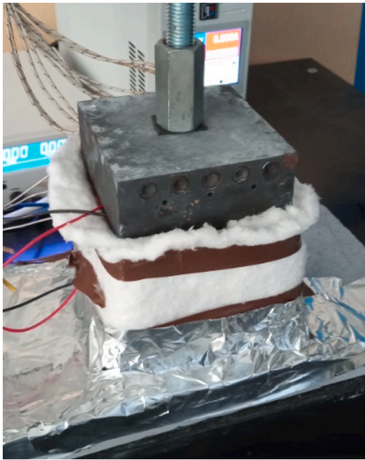
Fig. 3. Stand for experimental testing of the TEC in the sandwich configuration.
