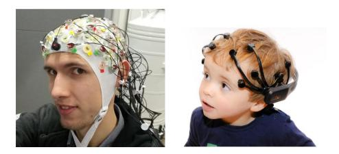
Figure 2-2. On the left: the BrainProducts actiCAP EEG cap with 64 electrodes (source: [25]). On the right: the Emotiv EPOC+ wireless headset with 14 electrodes (source: flic.kr/p/diA5hh).
