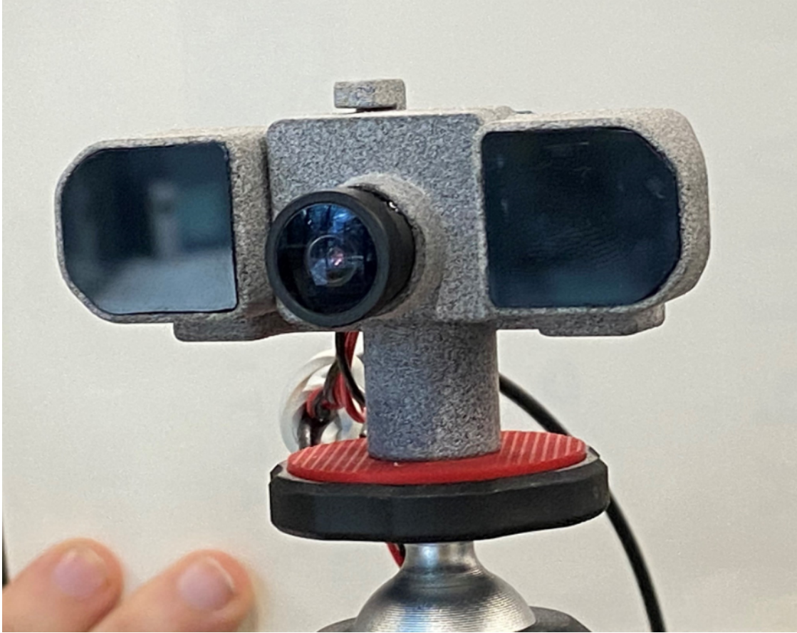
Figure 2.13: Example of RGB-IR interior sensing camera prototype with visible lens and active illumination concealed behind a covering glass.
