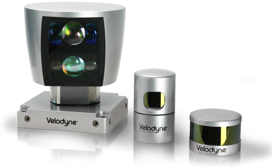
Figure 2.14: Examples of Automotive LIDARs - Velodyne LIDAR Family ( http://velodynelidar.com/ )
