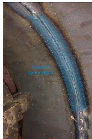
FIGURE 125: LACK OF PENETRATION ON GMA3 PIPE
