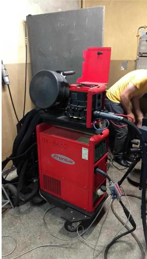
FIGURE 45: POWER SOURCE DEVICE FOR GMA APPLICATIONS
