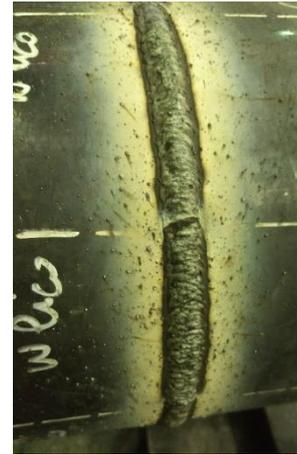
FIGURE 63: SSA4 SPECIMEN DURING MANUFACTURING PROCESS
