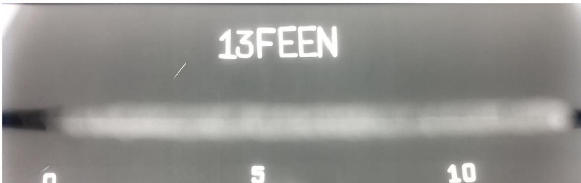
FIGURE 75: RADIOGRAPHIC TEST OF LASER ROOT PASS FOR COMBINATION 25
