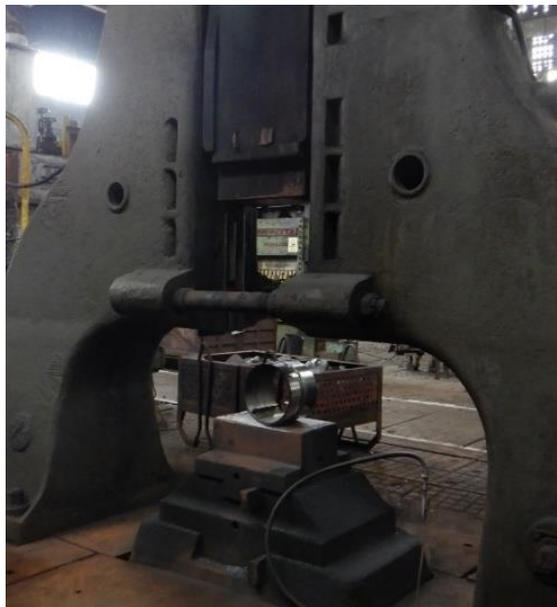
FIGURE 96: FORGING HAMMER SKM-3T
