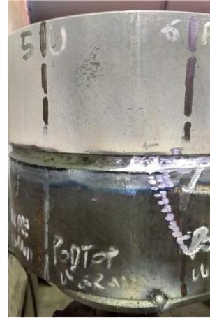
FIGURE 60: SSA1 SPECIMEN DURING MANUFACTURING PROCESS
