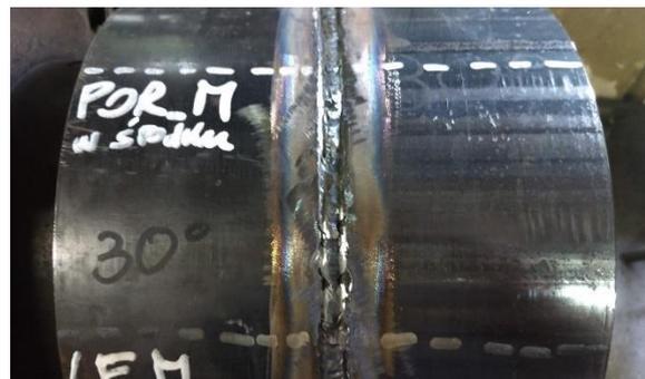
FIGURE 55: MMA2 SPECIMEN DURING MANUFACTURING PROCESS
