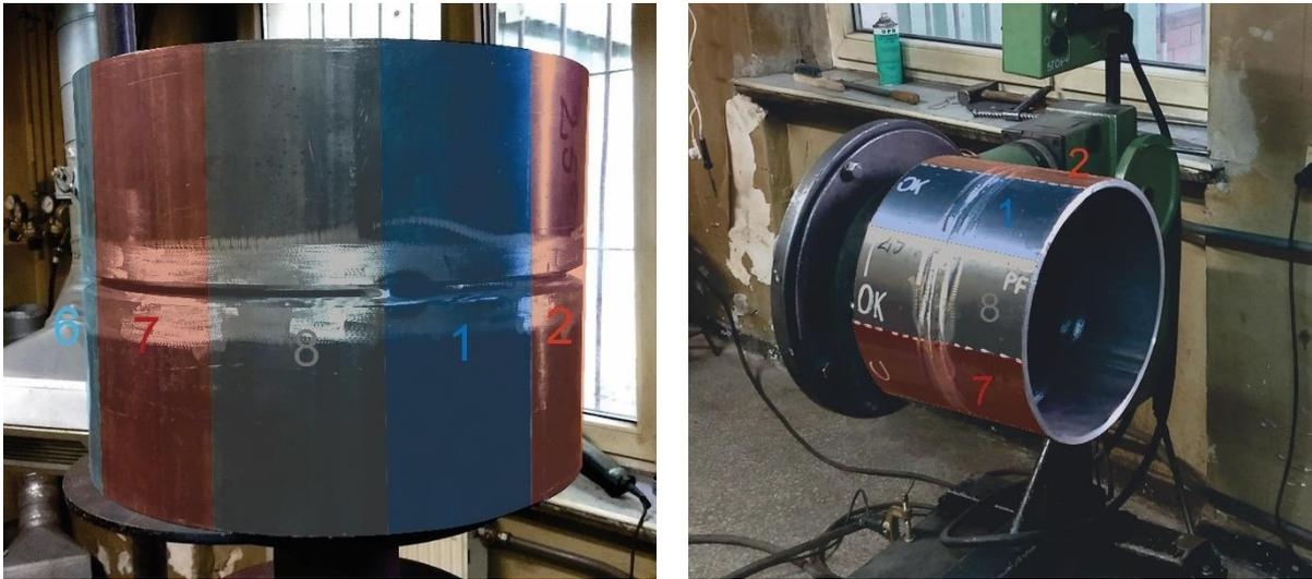
FIGURE 42: SEGMENTS ALONG THE PIPE CIRCUMFERENCE WITH DIFFERENT WELDING PARAMETERS APPLIED
