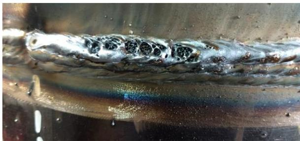
FIGURE 124: POROSITY ON GMA2 PIPE
