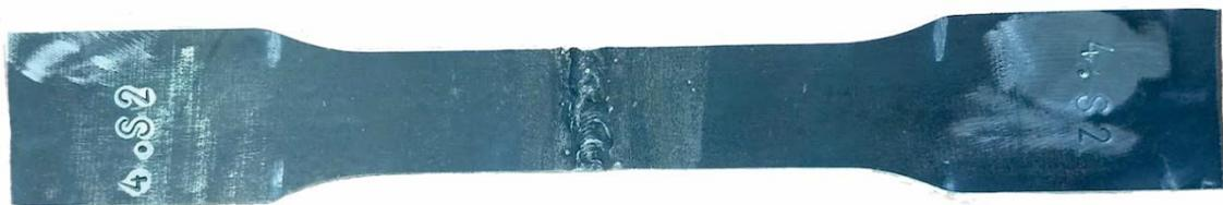
FIGURE 87: SAMPLE FOR TENSILE TEST OBTAINED FROM SSA PIPE
