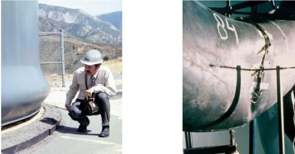
FIGURE 2: ELEPHANT FOOT BUCKLING OF A STEEL STORAGE TANK (LEFT) AND LOCAL BUCKLING OF A PIPE (RIGHT) [12]
