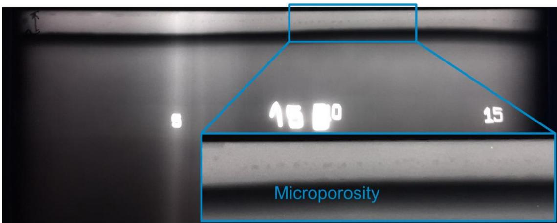
FIGURE 76: RADIOGRAPHIC TEST OF LASER ROOT PASS FOR COMBINATION 15
