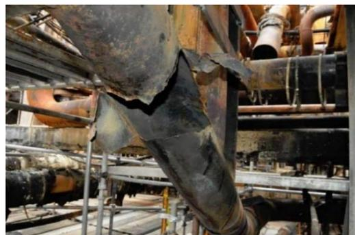
FIGURE 7: EXPLOSION AT CHEVRON REFINERY PLANT AND RUPTURE OF 52'' COMPONENT [16]
