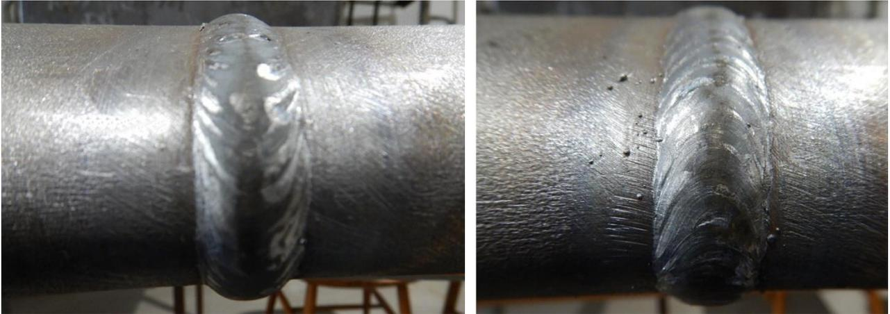
FIGURE 105: EFFECTS OF IMPACT LOAD TEST ON GMA PIPE SPECIMEN (1 M)
