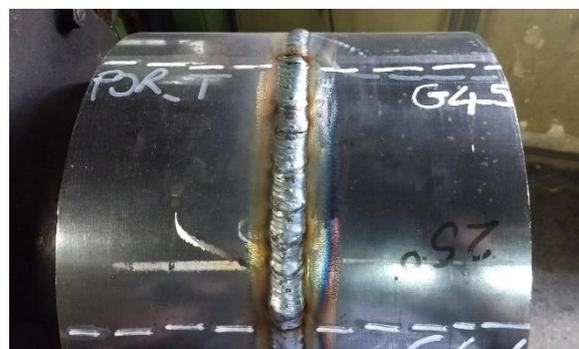
FIGURE 50: GMA4 SPECIMEN DURING MANUFACTURING PROCESS
