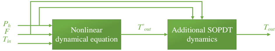
Fig. Ap4.3 The complete structure of the suggested model of the studied section of the heat distribution and exchange system.
