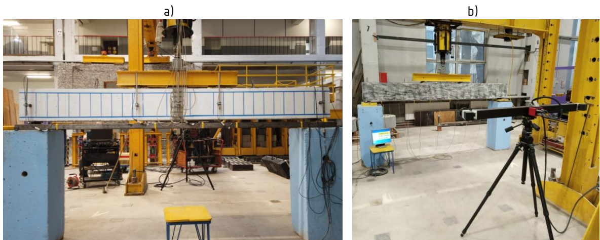
Fig. 3.4 a) Experimental setup of beam specimen on one side b) Measurement of the DIC system on the opposite side of the beam specimen
