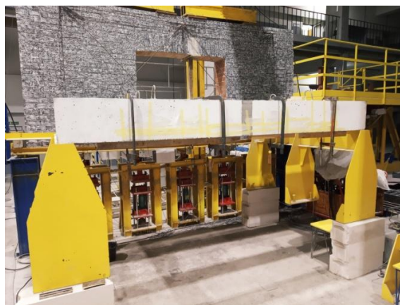
Fig. 3.8 Prepared specimen A6 right after CFRP application
