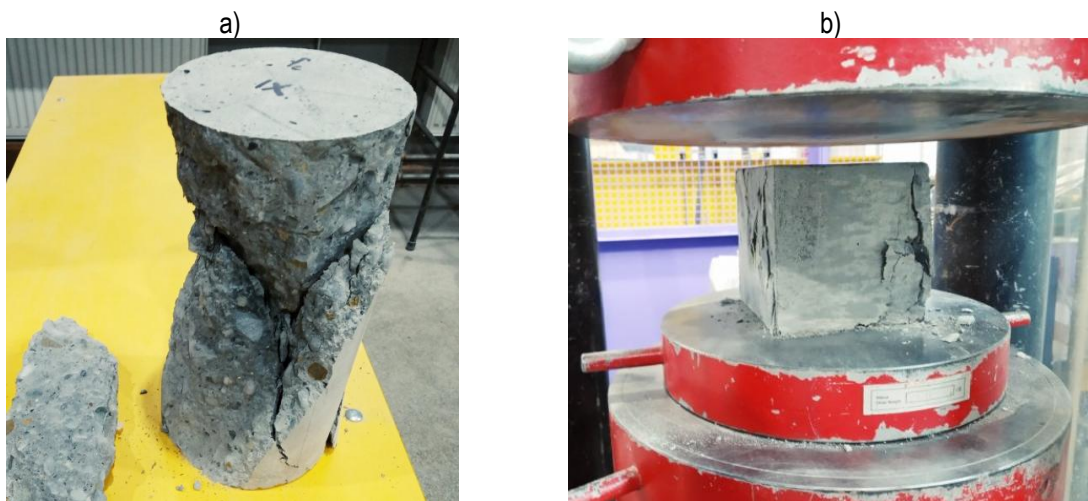
Fig. 4.9.: Typical failure mode of compressed samples: a) cylindrical b) cubic
