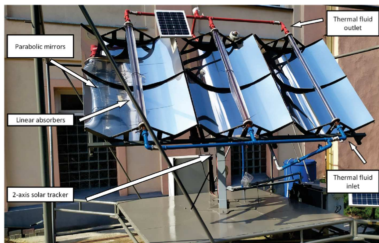
Fig. 1. Parabolic trough collector test facility with 2-axis solar tracker.
