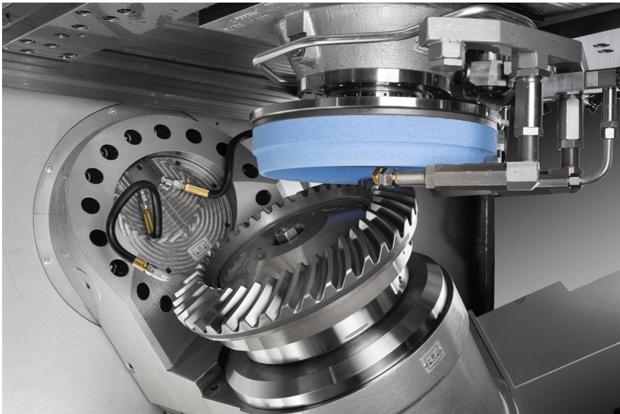
Fig. 1. Single indexing grinding on Klingelnberg G80
