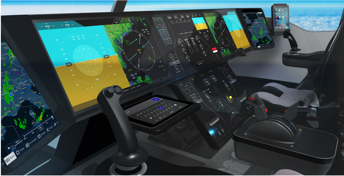
Figure 3.4: Future Systems Simulator’s cockpit close-up render. Every physical or digital element can be repositioned or removed according to research requirements.
