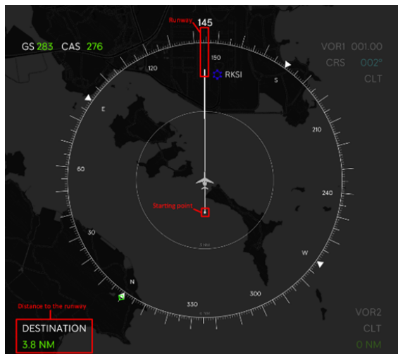
Figure 4.13: A visualisation from the pre-flight briefing of the second iteration of landing tasks, performed by participants 11+ in the main study (straight landing). During the descent, the pilot had to keep the aircraft aligned with the runway while maintaining the correct flight path. The figure shows the Navigation Display of the FSS, with task information marked in red.
