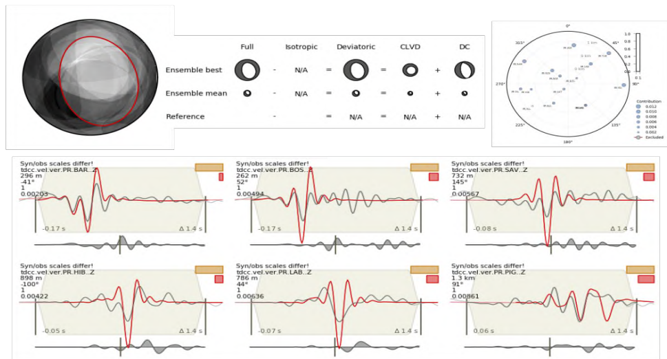
Fig. 7.6. Example of moment tensor inversion for a post-mining seismic event at Gardanne, France. The upper part of the figure shows the best moment tensor (red line) and range of acceptable solution (overlaid grey focal spheres), the moment tensor decomposition for the best and mean moment tensor solution, and the distribution of stations used in a polar plot. The bottom part of the figure provides some examples of data fit, comparing observed seismograms (black) and synthetic ones for the best moment tensor solution (red). The analysis was performed with the software Grond (Heimann et al. 2018)
