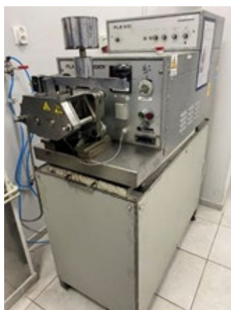
Rys. 4.36. Mikser laboratoryjny Brabender PlastiCorder Fig. 4.36. Brabender PlastiCorder laboratory mixer
