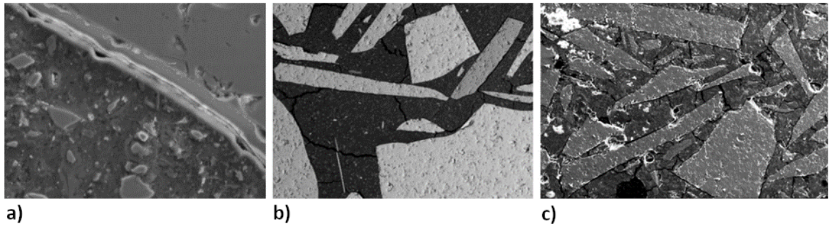
Fig.2.5.6: a) reaction on the surface between CRT particle and metakaolin, b) microcracks caused probably by improper amount of liquid, c) microcracks caused probably by too much CRT glass inside matrix [314].
