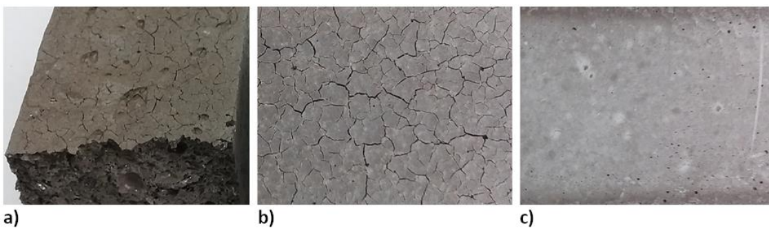
Fig.3.8.5: Samples cured at 20°C and demoulded after 24 hours (M/G 60/40): a) upper surface, b) side surface, c) bottom surface. Photos made after 7 days of curing.
