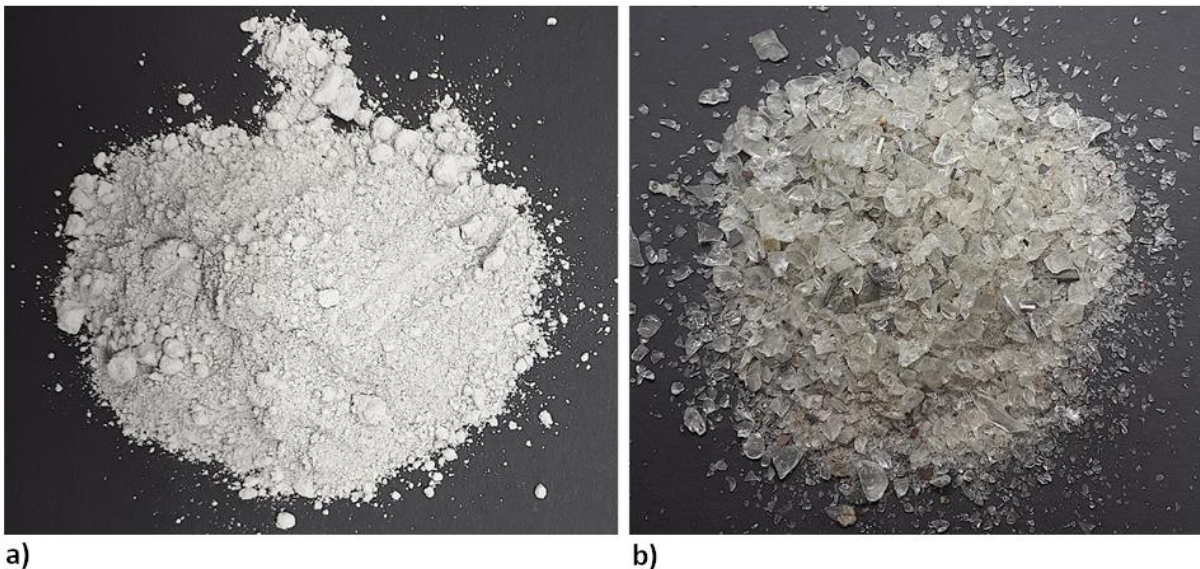
Fig.3.2.1: a) Metakaolin, b) CRT glass.
