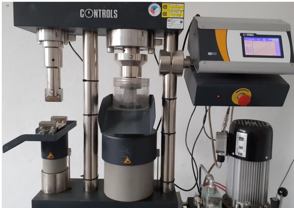
Fig.3.3.2: Strength tests machine Controls® Model 65-L27C12 Serial nr 12020060, during the compressive strength test.
