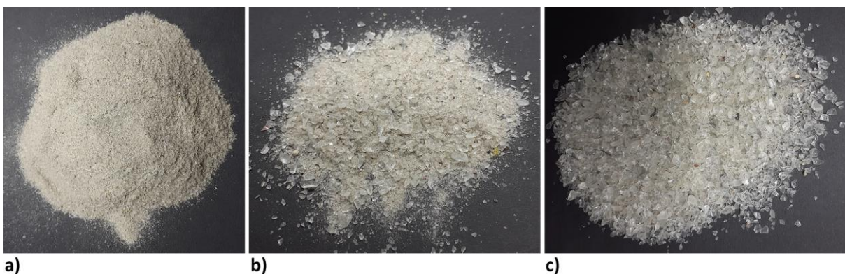
Fig.4.3.1: CRT glass of grain fraction a) < 0,5 mm, b) < 4 mm, c) 0,5 – 4 mm.
