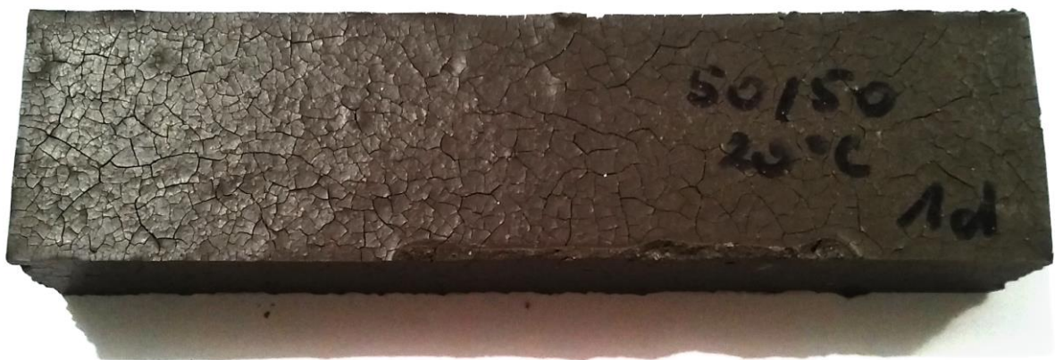
Fig.4.1.2: Sample cured at 20°C and demoulded after 24 hours. Picture taken after 27 days of further curing at the room temperature in the laboratory.
