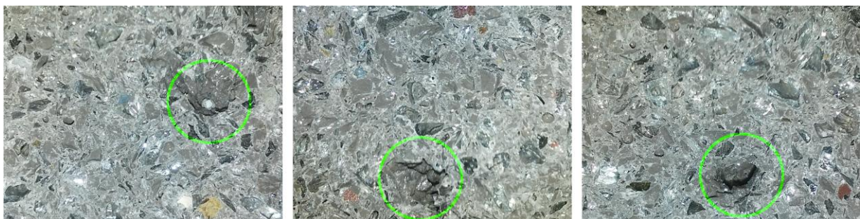
Fig.3.9.4: Cavities in geopolymer containing 75% of CRT glass. The biggest cavities were marked with the green circle.
