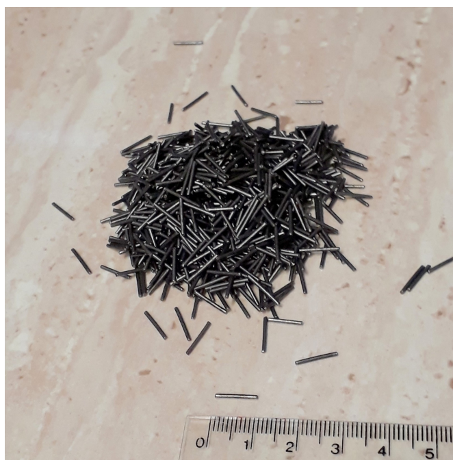
FIGURE 1.2: Standard grinding media for the EM mill: ferromagnetic rods of 10 mm length and about 1 mm diameter
