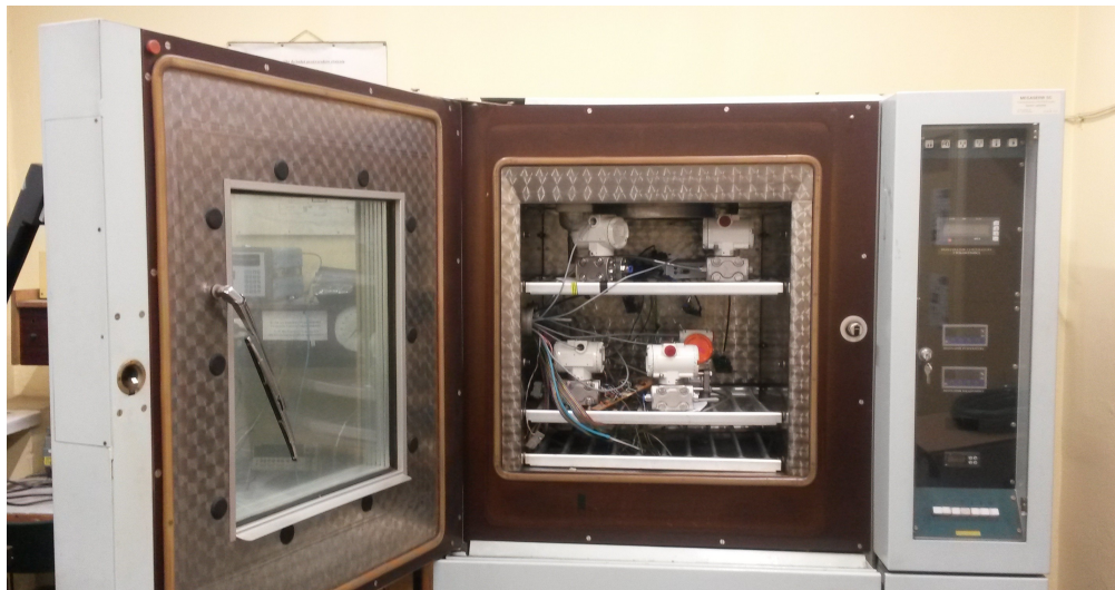
FIGURE 3.8: Pressure transducers inside climatic chamber
